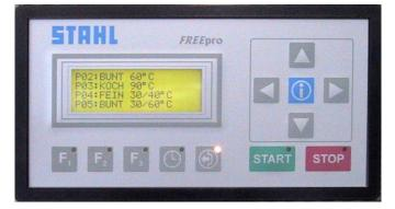
Our washer-extractors and drying tumblers are also controlled by the *FREE*pro. The advantage is that you can easily control three different procedures using one identical structure.
